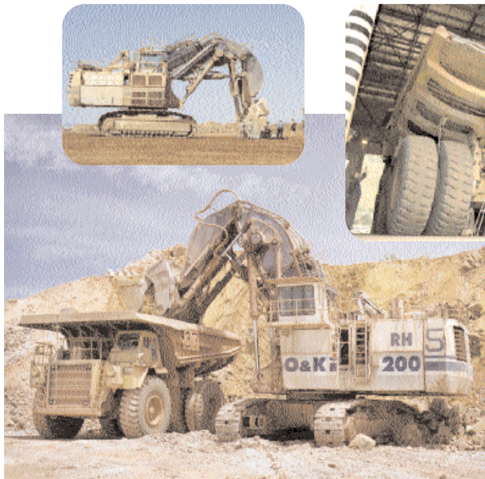
Figure 10. A mechanized shovel loads broken rock into a large truck for transport. The human figures in the insets provide some idea of the immense size of both the mechanized shovel and truck.
