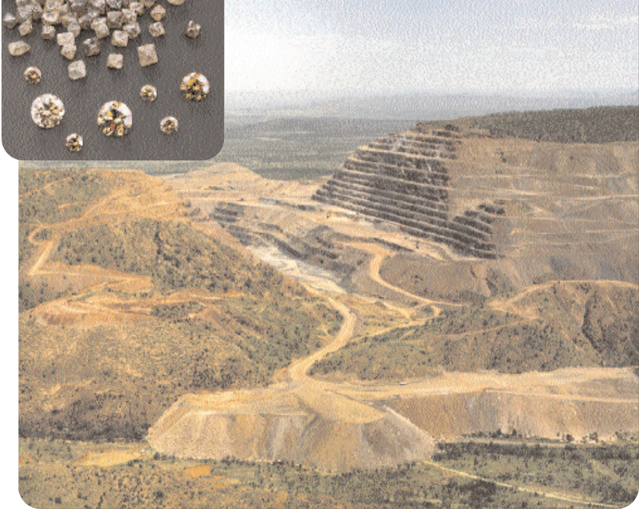
Figure 1. This aerial view of the Argyle mine, looking southwest, shows a portion of the AK1 pit. The shape of the open pit closely follows the outline of the lamproite pipe. In both the foreground and at the opposite end of the pit are dumps where the reddish brown overburden rock has been moved for storage. Since 1985, when mining of the orebody commenced, approximately 550 million tonnes of lamproite ore and overburden rock have been removed from the open pit. Brownish diamonds, such as the crystals and round brilliants shown in the inset, are commonly produced and marketed as “cognac” or “champagne” diamonds. The three largest diamonds weigh 4.11, 4.07, and 2.19 ct; inset photo by Shane F. McClure.
