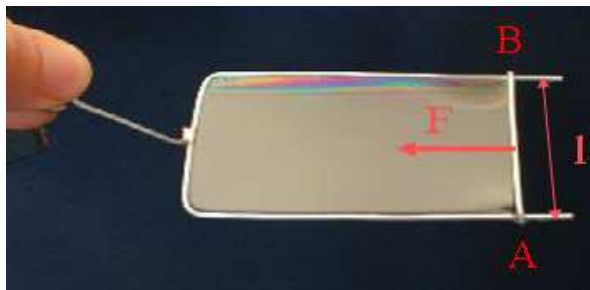
Figure 2: Soap bubble spanning the space inside the wire rim with a movable side AB.
