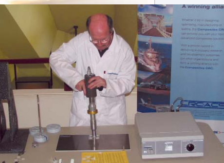
Above: Live demo on Ultrasonic Welding of Fittings to Composite Panels hosted by Daniel Bitton of the Composites CRC.
