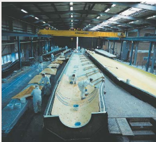
Above: Wet lay-up of wind turbine blades.
