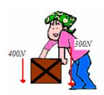
2. A modified peavey is used to lift a 0.2m diameter log of mass 3.6kg. Knowing that  $\emptyset$ =45 ° and that the force exerted at C by the worker is perpendicular to the handle of the peavey, determine the force exerted at C, (b) the reaction at A, [Beer and Johnston 2003, 189].
