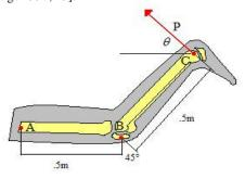
2. The man pulls on the cord with a force of 70 lb. Represent this force, acting on the support A, as a Cartesian vector and determine its direction, [Hibbeler 1986, 49].
