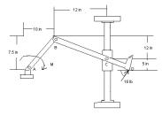
4. Determine the magnitude of the gripping forces exerted along line z-z on the nut when two 240-N forces are applied to the handles as shown. Assume that pins A and D slide freely in slots cut in the jaws, [Modified from: Beer and Johnston 2003, 338].
