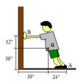
2. The coefficient of static friction between the person and the floor is **0.50** and the coefficient of static friction between the crate and the floor is **0.25** Determine the largest mass for the crate that the person can move by pulling on the cable if the person's mass is **70 kg**, [Ginsberg and Genin 1984, 12].
