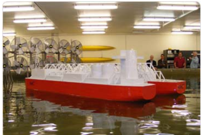
The gas-cat visualisation model being tested at the Australian Maritime College (AMC).
