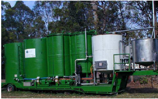
Initial Trial Mobile Batch Plant 2001 Design capacity 5000 l/day
