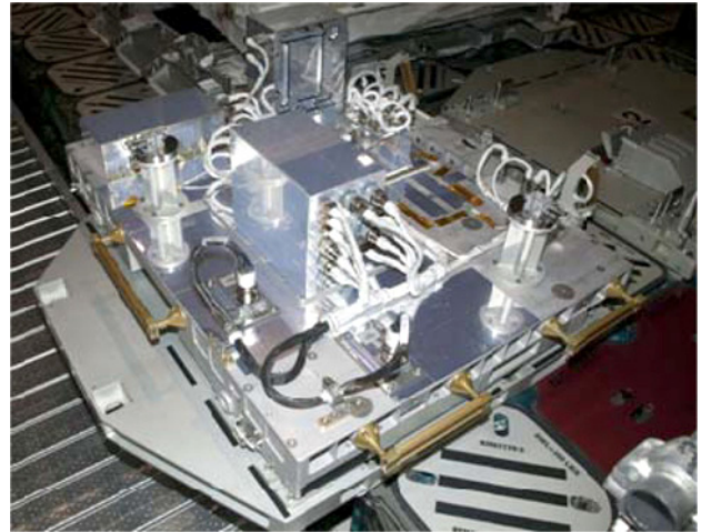
MISSE-7 Support Base installed on ELC2.
