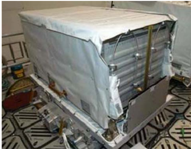
Nitrogen tank assembly installed on the ELC.
