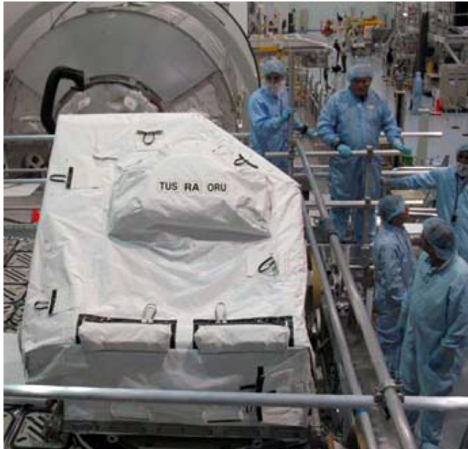
The trailing umbilical system reel assembly is shown in the space station processing facility at KSC.
