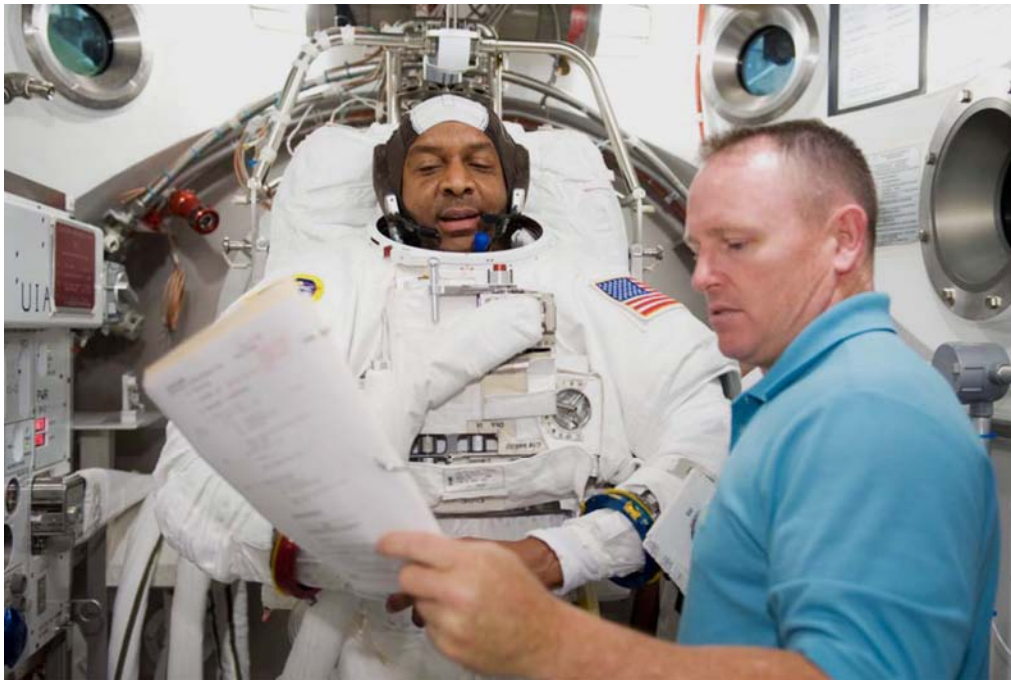
Astronaut Robert Satcher, STS-129 mission specialist, participates in an Extravehicular Mobility Unit (EMU) spacesuit fit check in the Space Station Airlock Test Article (SSATA) in the Crew Systems Laboratory at NASA's Johnson Space Center. Astronaut Barry Wilmore, pilot, assists Satcher.
