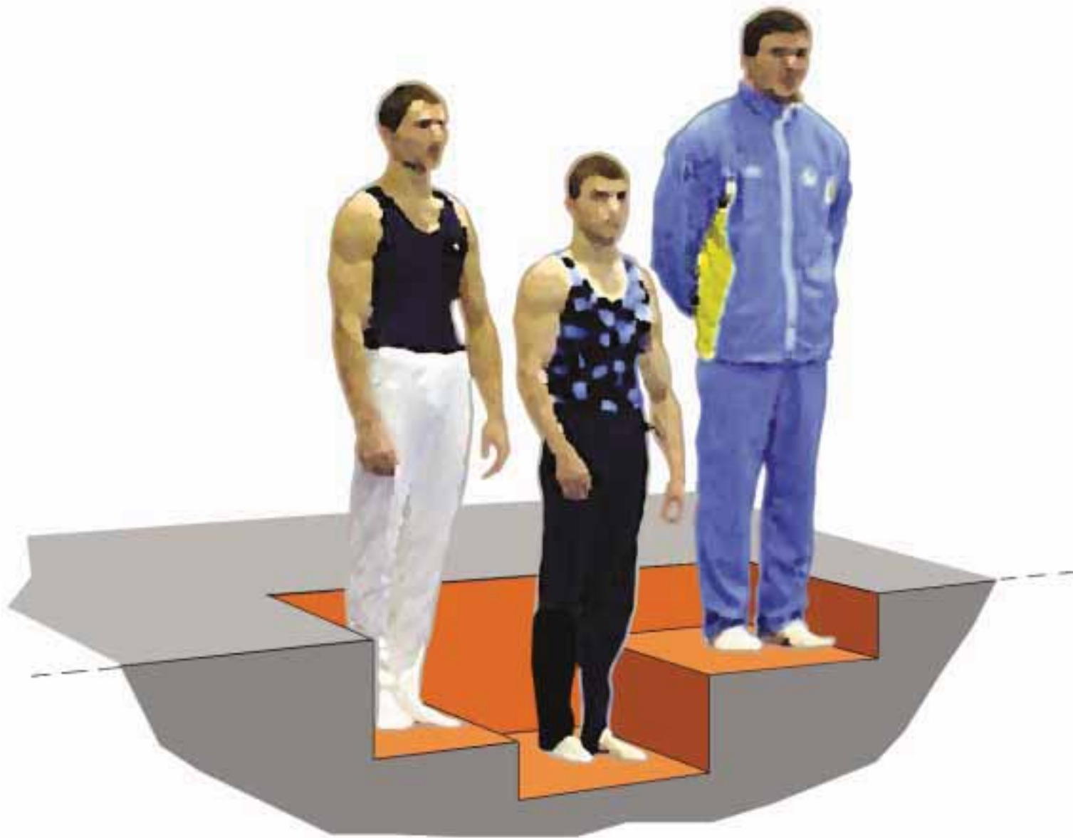
Inverted Rostrum (illustration) Sunken supawood installation. 80 x 240 x 80 cm
