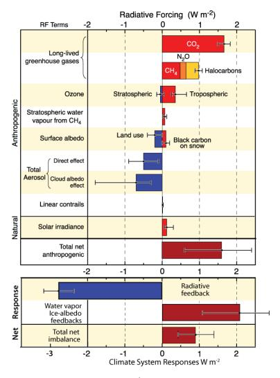
Fig. 4. The top part of the figure is the radiative forcing from IPCC<sup>1</sup> with the agents of change in left column and radiative forcing W m<sup>2</sup> with 90% confidence limits. The lower part shows estimates of the main negative radiative feedback, the water vapor, ice-albedo and other feedbacks, and the net radiative imbalance. Error bars for the latter are based on Fasullo and Trenberth<sup>7</sup> and others are approximate.
