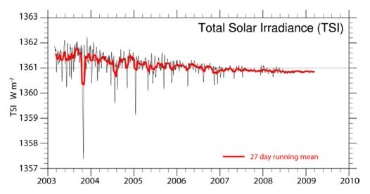
Fig. 5. Daily total solar irradiance from the Total Irradiance Monitor (TIM) instrument on the Solar Radiation and Climate Experiment (SORCE), along with a 27-day running mean in red. http://lasp.colorado.edu/sorce/index.htm (Data courtesy Laboratory for Atmospheric and Space Physics, U Colorado.)
