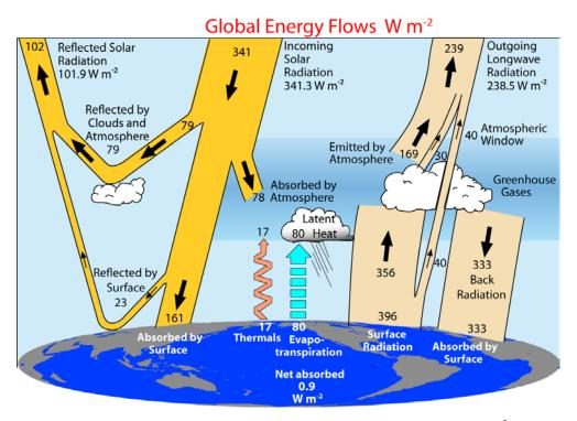
Fig. 2. The global annual mean Earth's energy budget for the March 2000 to May 2004 period in W m<sup>-2</sup>. The broad arrows indicate the schematic flow of energy in proportion to their importance. From Trenberth et al.<sup>6</sup>
