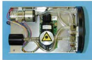
Optical Particle Counter Weight: 0.30 kg Dimensions: 96 x 60 x 34 mm Measure: size distr. 0.3 - 3 \mu m
