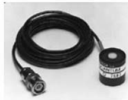
PAR radiometer Weight: 0.03 kg Dimensions: 24 \varnothing x 25 mm Measure: Irradiance 400 - 700 nm
