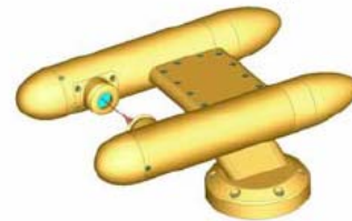
Cloud Droplet Probe Weight: 1.42 kg Dimensions: 216 x 115 x 100 mm Measure: drop size distr. 0.7 - 70 \mu m NOTE: electronics in fuselage
