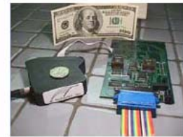
Spectral Radiometer Weight: NA Dimensions: 150 x 90 x 15 mm Measure: 350 - 1150 nm 256 channels
