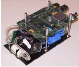
Condensation Particle Counter Weight: 0.87 kg Dimensions: 250 x 120 x 70 mm Measure: #/cc for D > 10 nm
