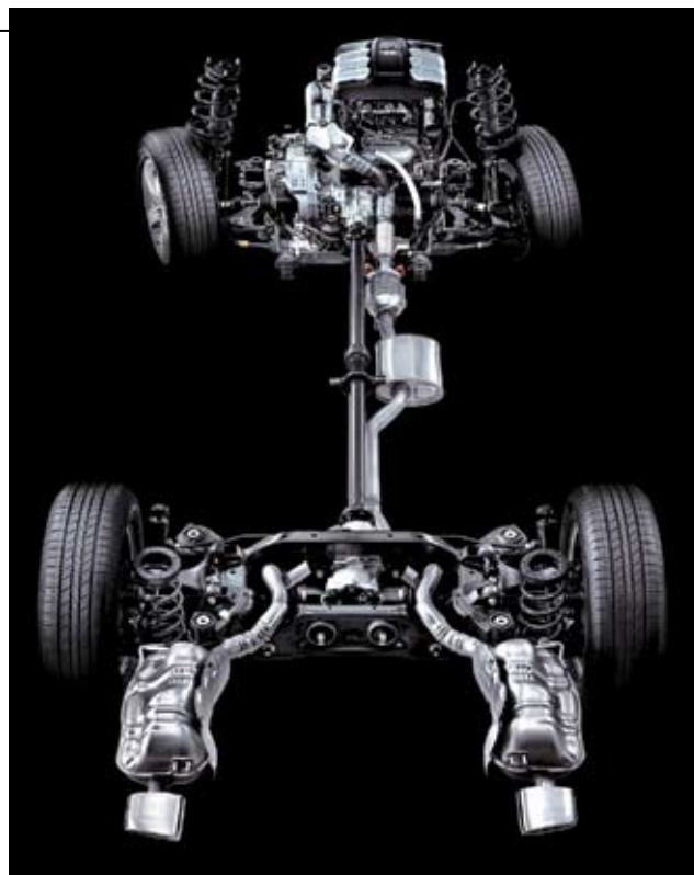
The S-Engine, shown here in the Veracruz chassis, is said to set new standards of refinement and performance for a diesel with its maximum output of 240 PS (237 hp/177 kW) at 3800 rpm and 46 kg-m (333 lb-ft) peak torque from 1700-3500 rpm.
