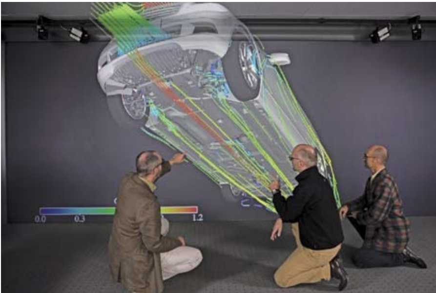
Using data from the digital prototype helped in developing the underbody aerodynamics of the C-Class.
