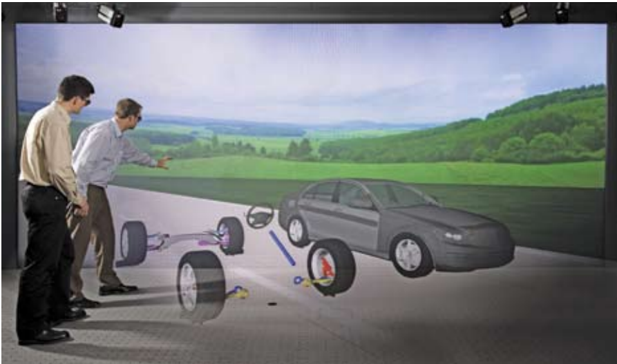
C-Class digital prototype "test driving" enabled fine-tuning of handling and ride characteristics.
