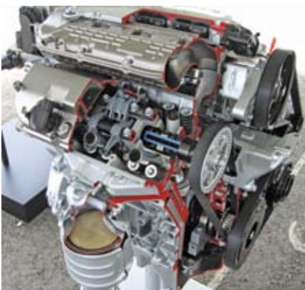
The MDX's 3.7-L VTEC V6 features a two-piece, dual-stage magnesium intake manifold and a drive-by-wire throttle system.
