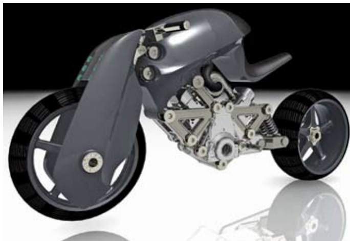
The Confederate Motors Renovatio will employ a girder-type fork and cast aluminum single-sided swing-arm mounting a pair of Penske Racing Shocks multi-adjustable dampers and Blackstone TEK carbon-fiber wheels.
