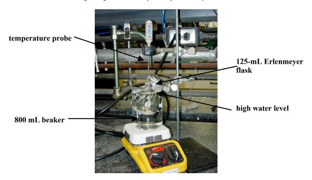
When you have the basic set-up accomplished, remove the flask. Place a boiling chip or two in the bath water and begin heating the bath. Dry the flask thoroughly. Cover the flask mouth with a small piece of foil and secure with wire or rubber band. Using a pushpin, make a pinhole in the foil cap. Measure (to the nearest 0.0001 g) and record the mass of the empty flask (w/ foil cap and wire).
