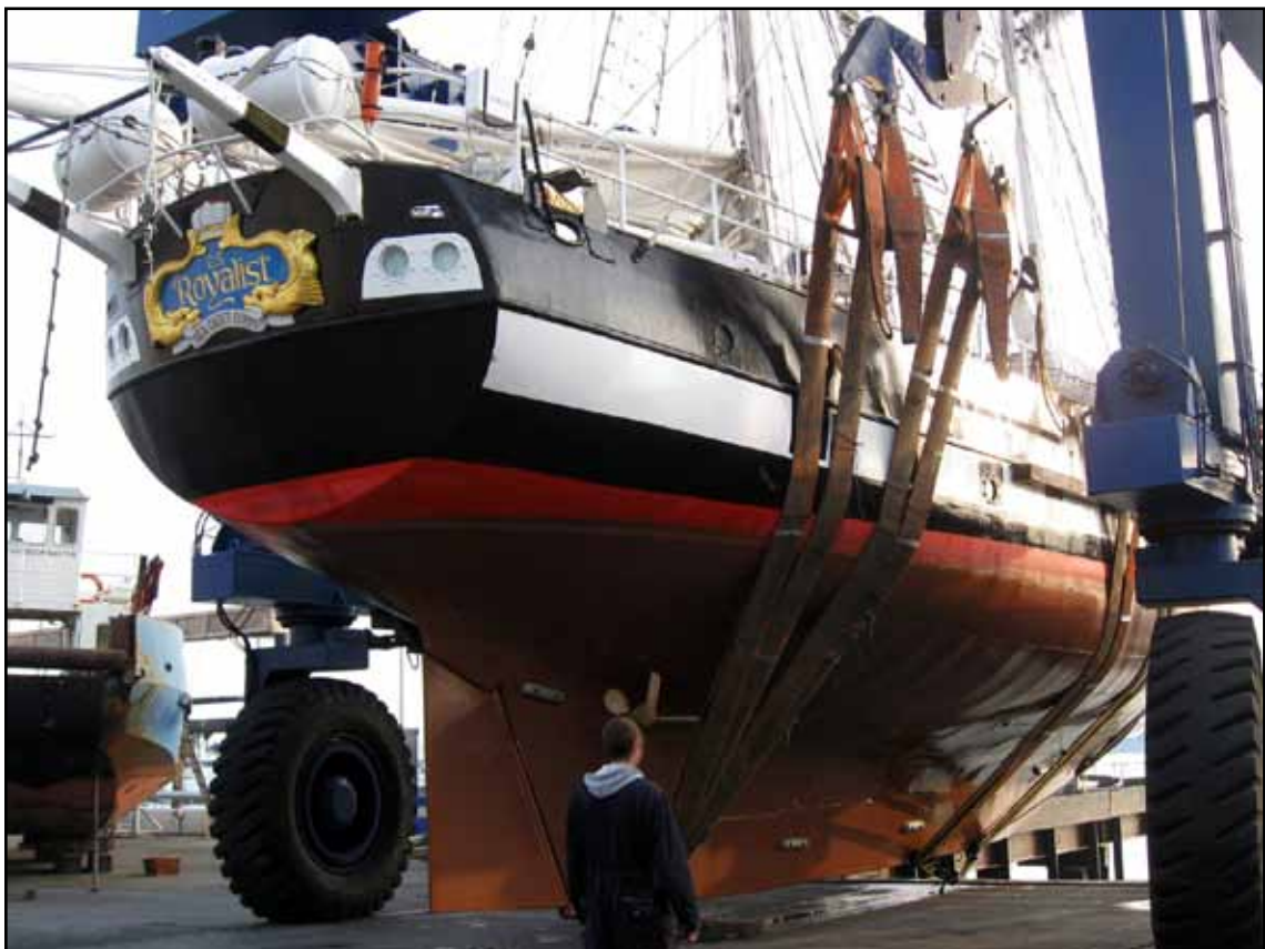
TS Royalist in the lifting cradle for hull inspection after the grounding
