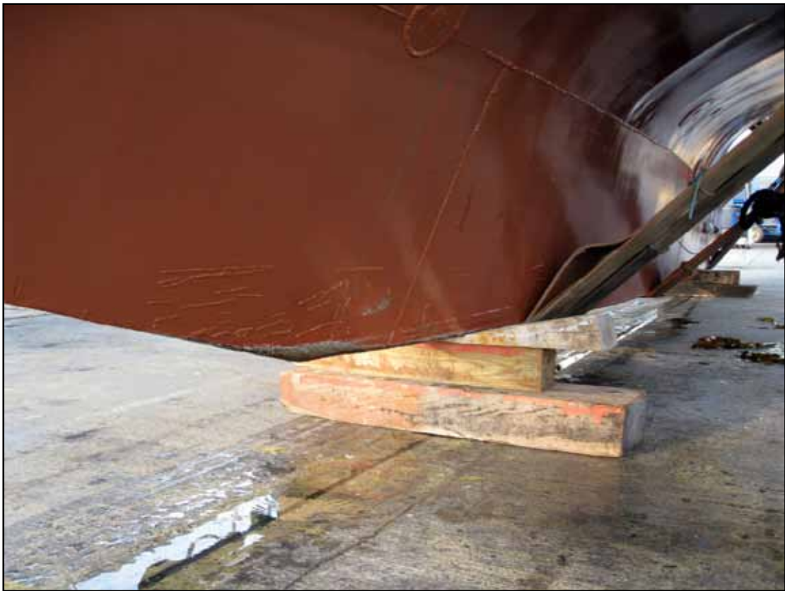
Minor scrapes to the anti-fouling of TS Royalist
