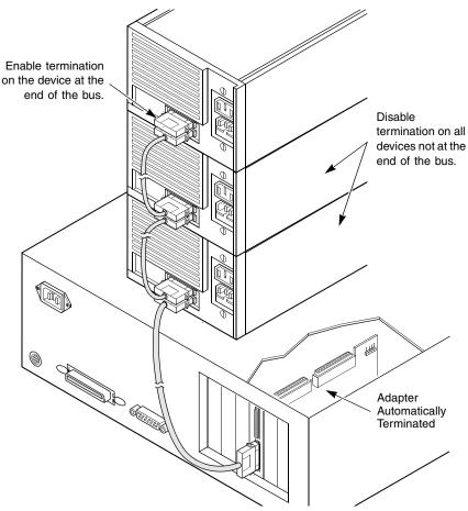
Figure 2.12 Connecting Multiple External SCSI Devices
