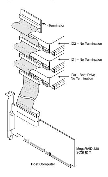
Figure 2.3 Terminating an Internal SCSI Disk Array
