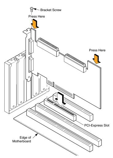
Figure 2.2 Inserting the MegaRAID 320-2E Card in a PCI-Express Slot
