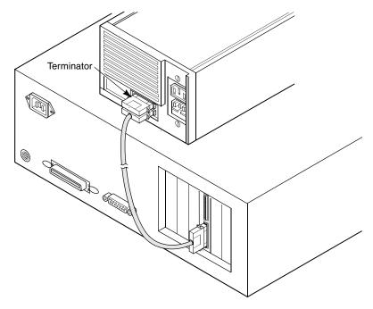
Step 3. Connect any additional SCSI devices to one another with shielded external SCSI cables. You need a separate SCSI cable for each additional device.
