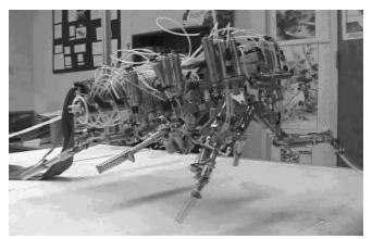
Figure 2. Robot III cycling its legs in tripod gait
