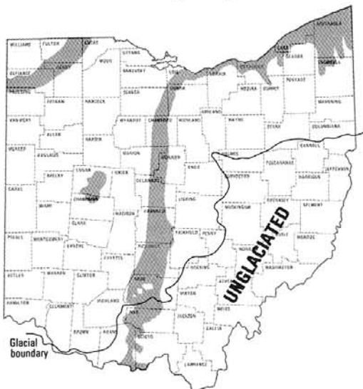
Outcrop area of the Ohio Shale in Ohio. In some portions of the state, north of the glacial boundary, the Ohio Shale is not exposed at the surface because of a thick mantle of glacial drift.
