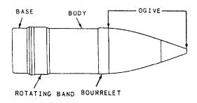
Figure 6-2.-Typical projectile, external view.
