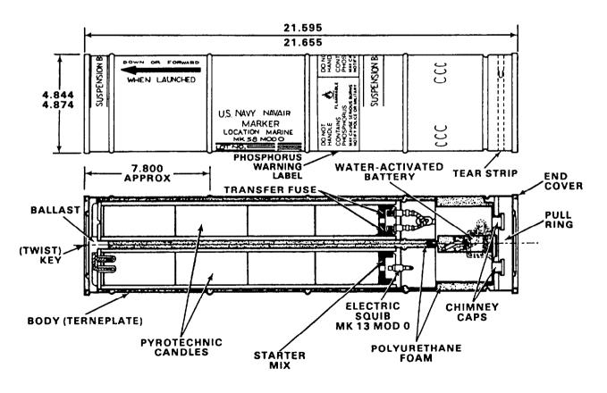
Figure 6-5.-The Mk 58 Mod 0 marine location marker.
