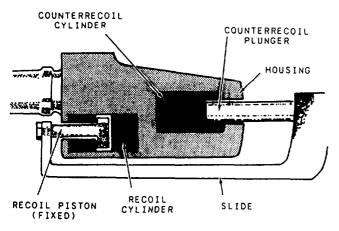
Figure 6-13.-A basic recoil and counterrecoil system.
