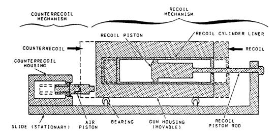
Figure 6-12.-Recoil and counterrecoil system.
