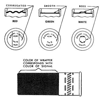
Figure 6-8.-The Mk 2 marine illumination signal.
