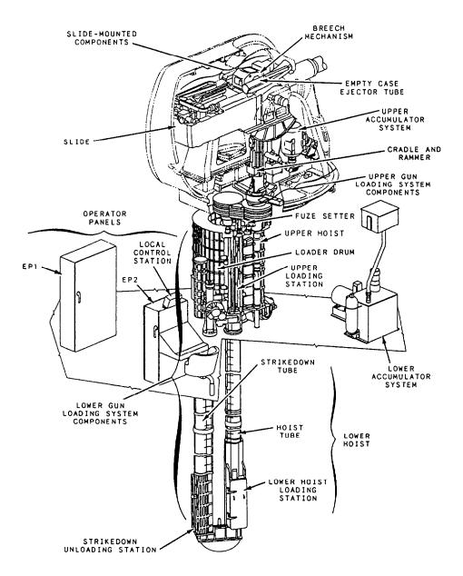
Figure 6-17.-The 5"/54 Mk 45 gun loading system, major components.
