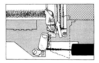
Figure 6-11.-The sliding-wedge breechblock.
