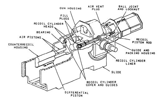
Figure 6-14.-5"/54 Mk 42 recoil and counterrecoil system.
