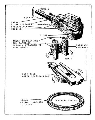
Figure 6-10.–Gun-positioning equipment.
