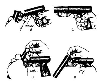
Figure 6-9.-Operation of the Mk 5 pyrotechnic pistol.
