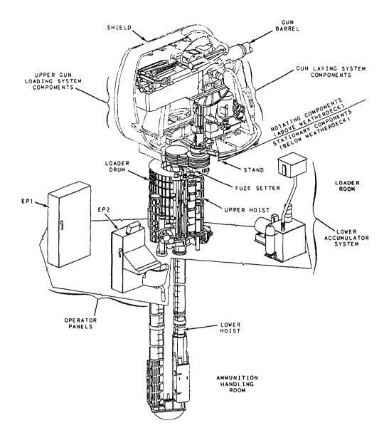
Figure 6-16.-The 5"/54 Mk 45 Mod 0, general arrangement.
