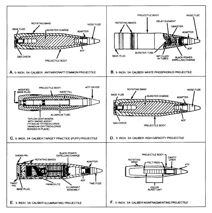
Figure 6-3.–Common projectile types.
