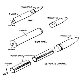
Figure 6-1.—Types of gun ammunition: fixed (top); semi-fixed (center); and separate-loading (bagged gun) (bottom).
