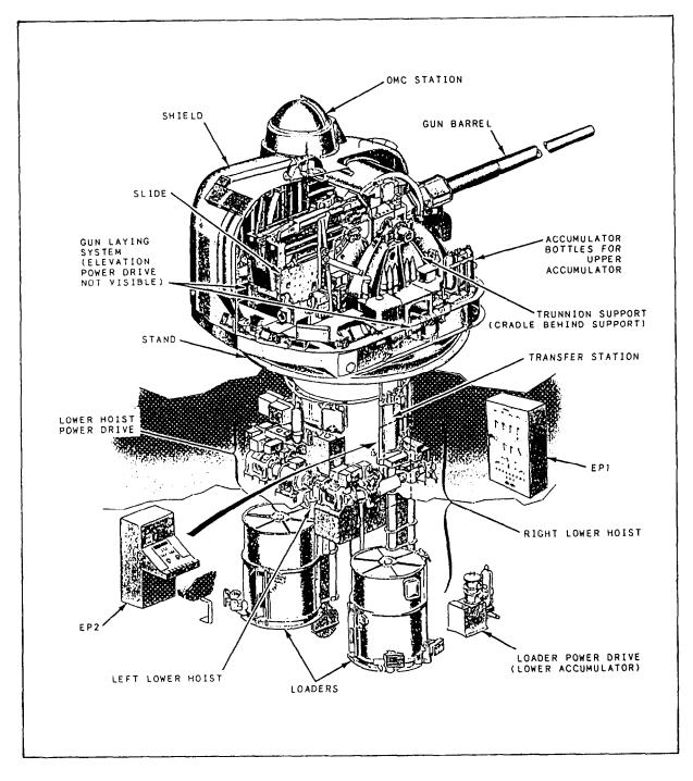
Figure 6-15.-Major components of the 5"/54 Mk 42 (Mod 10 shown).
