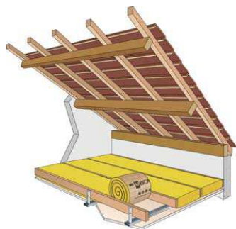
Insulation between rafters
