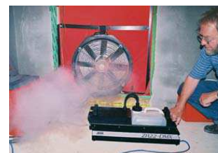
Air leak test with artificial smoke and overpressure
