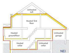
Parts of the heat-transmitting envelope
