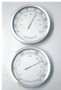
Mechanical temperature and humidity meters
