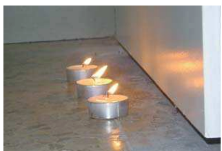
Candles make cold airflows visible
