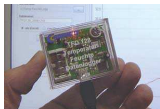
Small electronic temperature and humidity data logger with USB connection to computer
