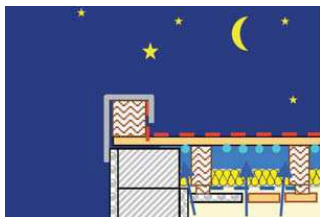
Condensed water forming on the bottom surface of an upper boarding installed on a flat cold roof when exposed to cold night temperatures
