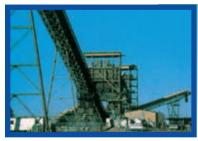
**COAL CONVEYORS:** After retrieval from the storage area by the stacker-reclaimer, coal is transported into the boiler building on a coal conveyor system that's enclosed to control dust.
