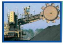
**COAL STACKER-RECLAIMER:** Coal is stored and retrieved by a bucket-wheel, stacker-reclaimer, which moves within the coal yard on a set of railroad tracks.
