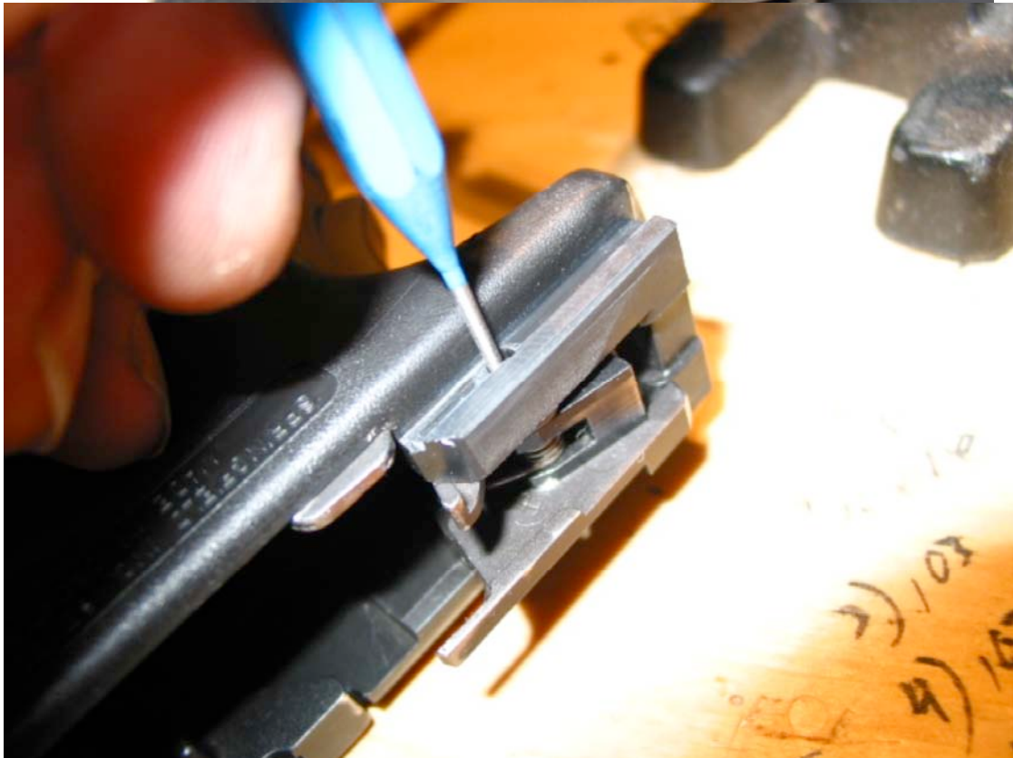
Lightly tap the punch (a 1/16 inch punch is all you need to take down the entire gun to remove this pin.
