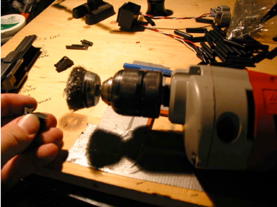
I polished off the black oxide with a wire brush chucked in a drill.
