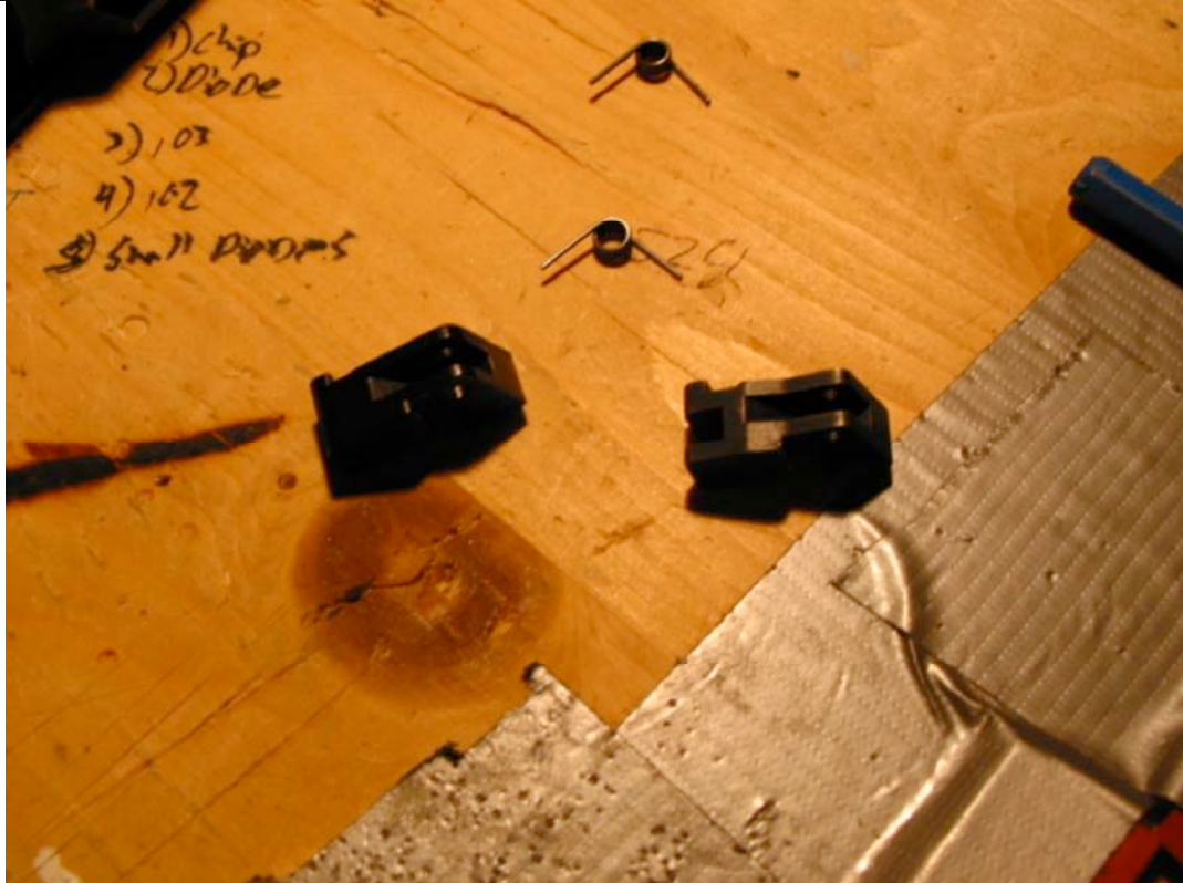
The replacement Sear, and Sear spring. The Replacement Sear is also black oxidized.
