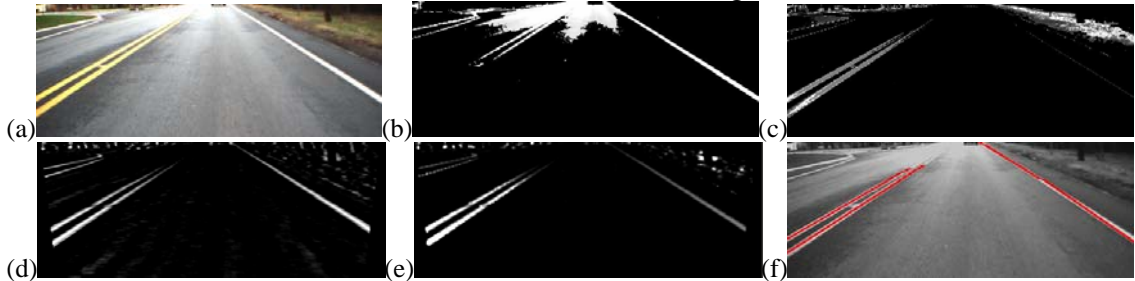
Figure 6: Stages of Lane Detection (a-f).
