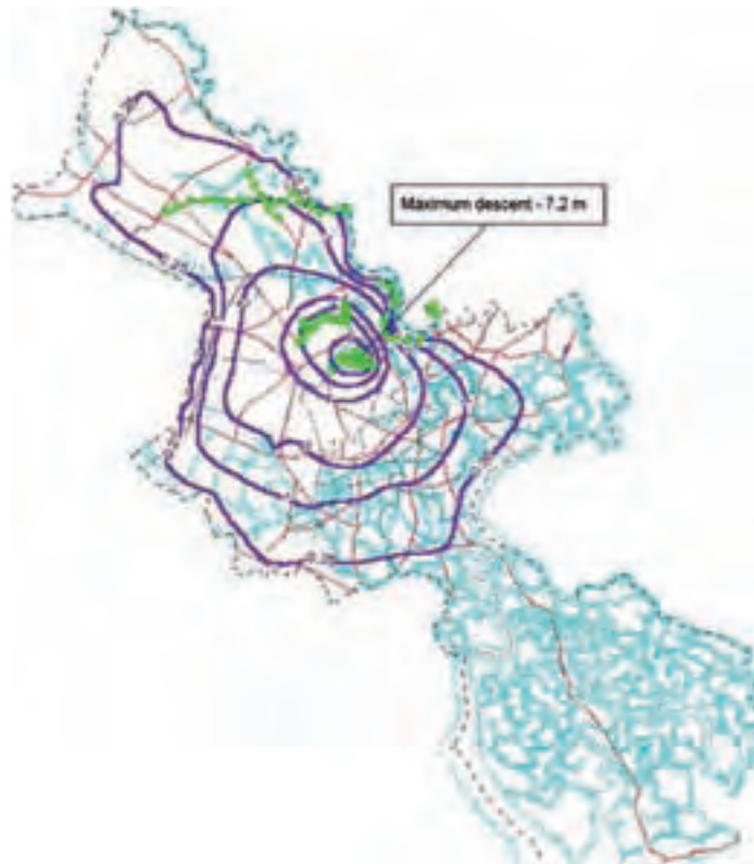
Figure 4. Water Table Drawdown of Upper Pliocene – 2010 in Comparison to 2001 Source: DI, 2002
