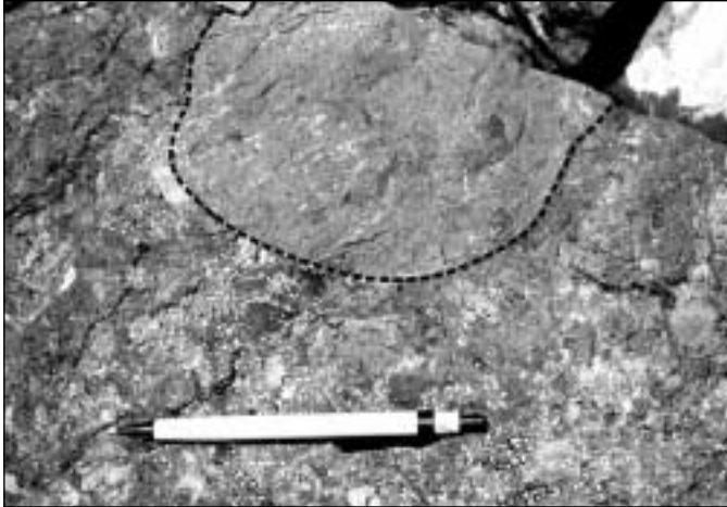
Figure 30. Well-rounded cobble-sized clast of altered siltstone of the Wernecke Supergroup in Wernecke Breccia, Olympic mineral occurrence (Yukon Minfile, 1997).
