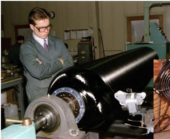
Graphite-Epoxy Composite Case Winding (21-in. booster)
