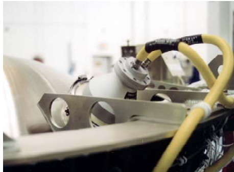
CSC Installed on Lunar Prospector TLI Stage
