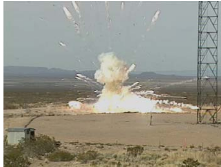
STAR 48 Destruct Test Using Model 2011 CSC
