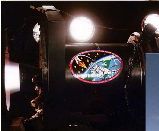
Motor Static Firing at Simulated Altitude (ASAS AKS-2 Qualification Motor)
