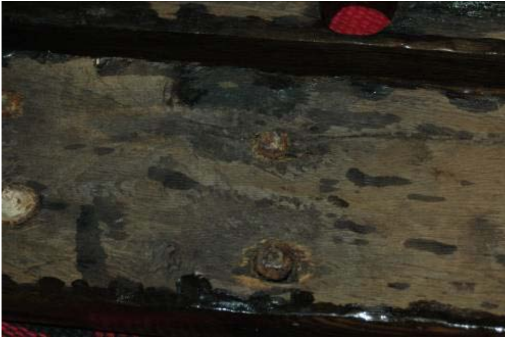
Figure 7.2: Unpreserved under side of coffee table note the Iron peg heads (C. Golden Photo)
