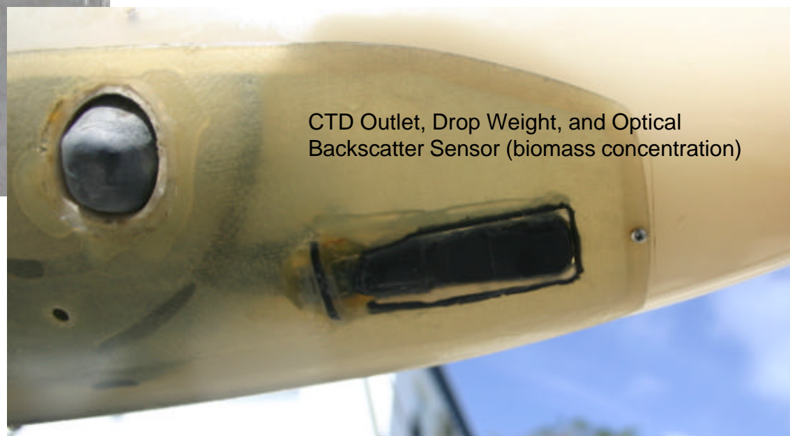
CTD Sensor: Temperature Salinity (conductivity) Pressure
