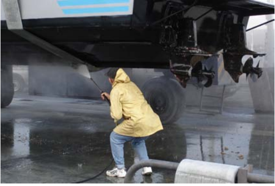
Figure 1: Initial removal of fouling epibiota by water blasting at Tauranga Marina (A) and Lyttelton dry dock (B).
