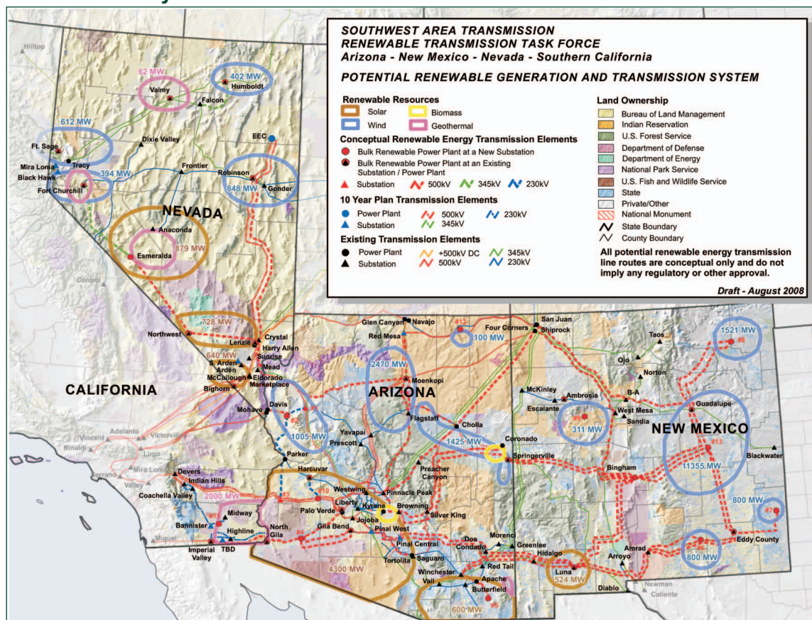
Figure 3-2. SWAT Renewable Energy Zones and Current and Potential Transmission System
