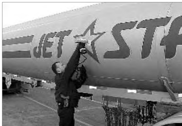
A US Customs inspector uses CHAIS to identify a tank's contents.
