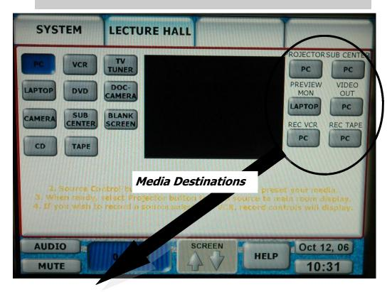
**Projector:** Source media will display through the projector **Sub Center:** Source Media will display in the Sub Center Rm# 113 **Preview Monitor:** Source media will display in the preview monitor located at the back of the lecture hall (this monitor is not visible from the
