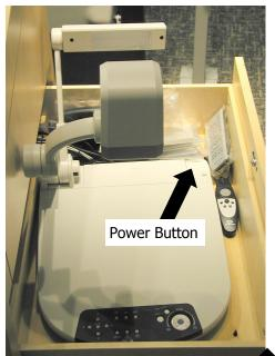
The document camera is located on the side of the lectern. Unlock the side panel, and slide out the document camera drawer. Lift the light and head of the document camera. The camera can display any type of object (photos, coins, papers, etc).
