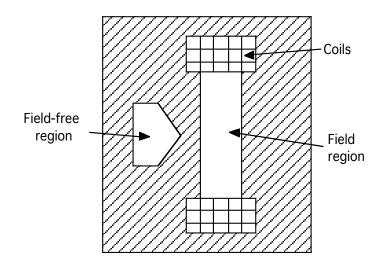
**Lambertson**. This magnet has two apertures: a magnetic field region (like a dipole), and a field free region. It's used as an injection or extraction device in circular accelerators or as a way to separate beams in a beam line.
