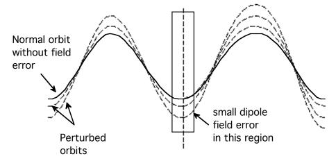
In reality, we do not simply have one imperfect magnet with a dipole field error. Every magnet in every accelerator can be considered to be slightly flawed. Even if all of the magnets were perfect, slight misalignments could generate these types of incorrect fields as well. Because of dipole field errors, the tune of any accelerator cannot be equal to 1, or in fact equal to any integer value.
