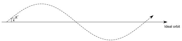
**Position and angle**. A particle's trajectory at any point can be described in terms of its distance from the design orbit, x, and the angle between its trajectory and the ideal orbit, x'.
