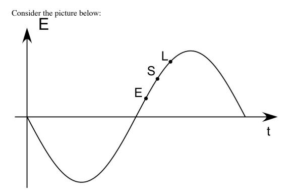
**Acceleration**. The sinusoidal curve represents the magnitude of the accelerating electric field in a RF cavity versus time. The labeled points represent various beam phases.
