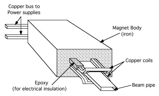
Specially treated cooling water (called LCW, which stands for Low Conductivity Water) flows through the passage inside the bus to carry away the large amounts of heat generated by the high current flow. Also notice that an iron magnet body, which concentrates and shapes the magnetic field, surrounds the coils. Finally, notice how the beam pipe inside the magnet is placed very close to the coils themselves. This maximizes the magnetic field "felt" by the beam passing through.
