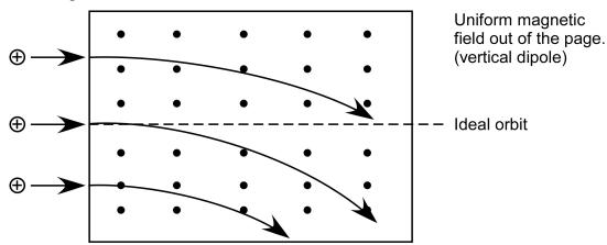
Attempt at vertical focusing. The three arrows at the left represent three different particles within a bunch. The top most is the imperfect particle in the example in that has drifted upwards. The center arrow is a perfect particle initially traveling on the design orbit. The bottom arrow is another imperfect particle that has drifted downwards. When all three particles enter the field created by the vertical dipole, they are deflected downwards.
