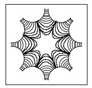
**Octupole magnet**. The octupole has eight magnetic pole faces. The lines indicate magnetic fields. It controls the coupling between betatron tune and betatron oscillation amplitude in an accelerator.
