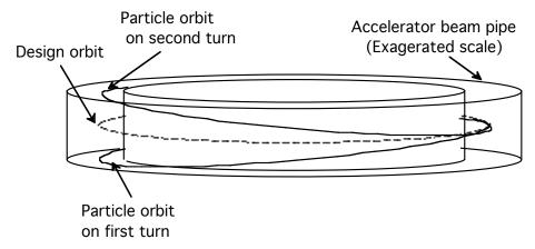
If a particle has a fractional tune value of 0.5, the same trajectory is traced out every other revolution in the accelerator. If there is a dipole error at some point, like in the example above, on one revolution the particle will see a kick to increase the oscillation. On the next pass through the region, however, the same kick would tend to reduce the oscillation. See below:
