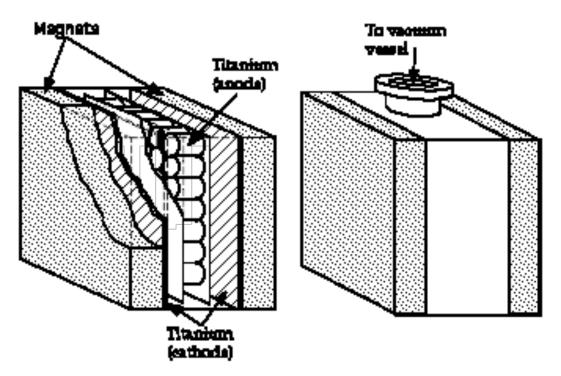
**Ion Pumps**. This pump works by ionizing air molecules then capturing the free electrons on the anode and the ionized molecules on the titanium plates. An electrical current proportional to the number of ions created can be measured, indicating the quality of the vacuum. Molecules trapped in this way no longer contribute to the vacuum pressure inside the beampipe.
