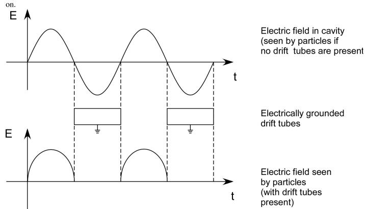
**Electric fields with drift tubes**. The graph on top represents the magnitude of the accelerating electric field in a RF cavity versus time. The bottom graph shows only that portion of the electric field seen by particles in a cavity equipped with drift tubes.
