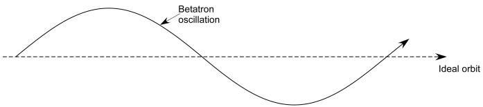
**Betatron Oscillations**. Quadrupole focusing forces particles into transverse oscillations about the ideal orbit. The particle's path is shown as the solid line above.
