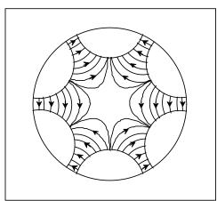
**Sextupole magnet**. The sextupole has six magnetic pole faces. The arrowed lines indicate magnetic fields. A sextupole controls the chromaticity in an accelerator.
