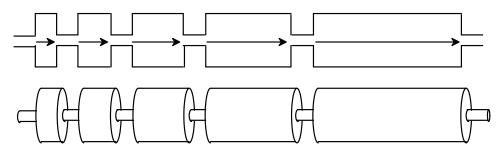
Constant Frequency with an Increasing Acceleration Gap Length
