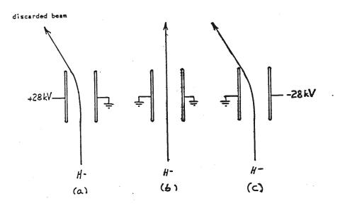
**750 keV chopper** – .The chopper is made up from a pair of conducting plates that straddle the beam path, allowing a portion of a more or less continuous stream of charged particles to be deflected.
