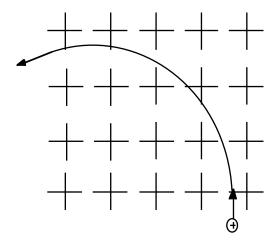
**Bend Field.** The crosses indicate a magnetic field pointing into the page. Given the positively charged particle initially traveling upwards, the right hand rule dictates a force to the left, deflecting the particle from its original path.
