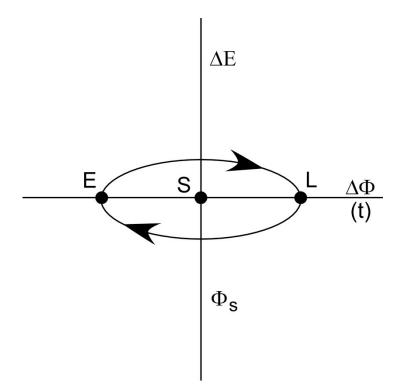
**Phase Space Diagram**. Here is a good way to view synchrotron oscillations—phase errors become energy errors become phase errors and so on. The labeled points represent various initial beam phases.
