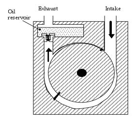
**Roughing Pump**. This pump has rotating vanes that trap air molecules and mechanically force them out the one-way exhaust valve.
