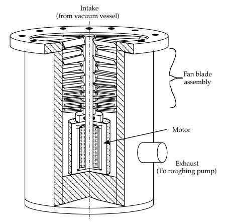
**Turbo pump**. This pump acts like a turbocharger for the roughing pump. Spinning vanes deflect molecules down toward the exhaust port and the connected roughing pump.
