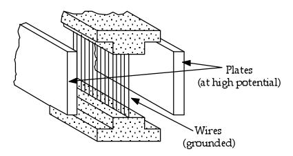
**Electrostatic Septa**. Beam travels between the high voltage plates and is split into two separate beams. The electric fields formed between the conductive plates and the grounded wires provide the force for this splitting effect.
