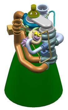
Colo., and Concepts NREC of White River Junction, Vt., has designed a single shaft main turbopump. This turbopump includes long-life hydrostatic bearings and a pressurized interpropellant seal cavity, offering a higher safety margin by helping to keep the propellants separated. Other attributes of the TR107 engine are advances with the oxygen-rich preburner, including a single pintle injector and oxygen-compatible materials that eliminate the need for coatings on engine components.
