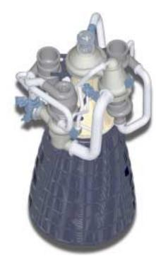
wall nozzle offer increased efficiency, lower heat loads, and longer life. The RS-83 uses low-torque, innovative cartridge-style valves to increase operability, reduce weight, and minimize leak points. The engine will offer a minimum lifespan of 100 missions and a maintenance check-up every 50 missions.
