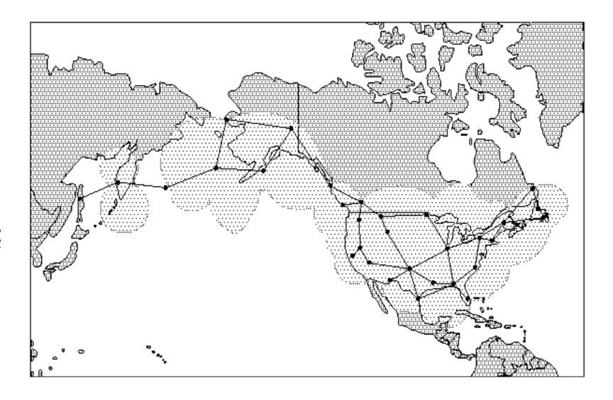
Figure 3-5. Coverage Provided by U.S. or Supported Loran-C Stations
