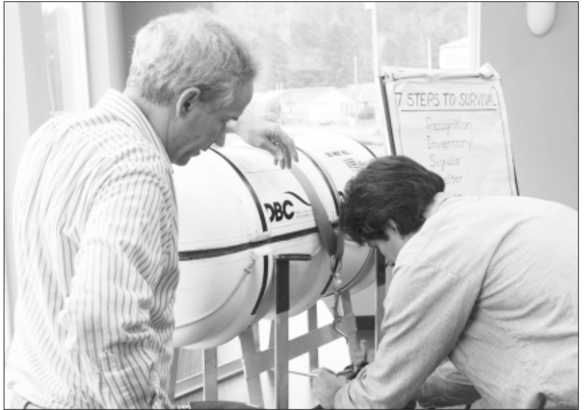
Steve Harbell, left, works with a fisherman who is learning to properly hook up the hydrostatic release on a life raft. (Photo courtesy of Steve Harbell, WSU Gray's Harbor)
