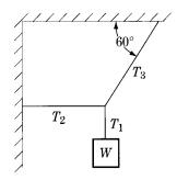
4. A system in equilibrium consists of an object of weight W that hangs from three ropes, as shown above. The tensions in the ropes are  $T_1$ ,  $T_2$ , and  $T_3$ . Which of the following are correct values of  $T_2$  and  $T_3$ ?
