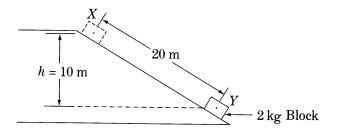
A 2 kg block, starting from rest, slides 20 m down a frictionless inclined plane from X to Y, dropping a vertical distance of 10 m as shown above.
