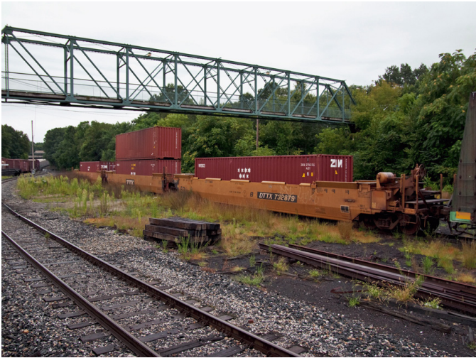
This image shows the first Connecticut double-stack container, operated by RailAmerica, Inc. Increased vertical clearances enable double-stack containers, which increase shipment volumes.
