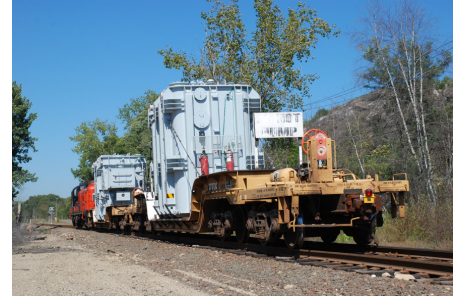
This image shows the relationship between the freight rail network and the regional electric grids. NAUG is hauling over-dimension and over-weight electric transformers to Northeast Utility's Watertown Substation, which feeds Fairfield County. Repairs and improvements to the network are imperative to ensure the ability to move over-size loads.
