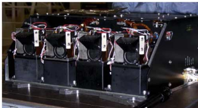
Figure 1. Photograph of the MECA instrument package showing the placement of the four WCL units just prior to integration onto the Phoenix spacecraft deck at Lockheed Martin.
