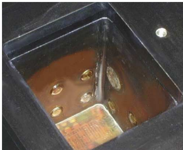
Figure 8. View of the sensors on two of the walls inside the WCL beaker.
