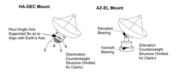
HA-DEC antenna mounting systems require an asymmetrical structural design unsuited to the support of very heavy structures. Their advantage is that motion is required mostly in only one axis to track an object as Earth rotates, although this advantage has largely been obviated by the use of digital computers that can drive both axes of AZ-EL systems properly while they track. The GAVRT uses an HA-DEC mount.
