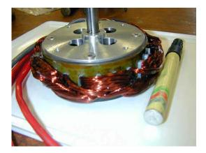
Fig 6 100 mm od. axial flux machine
