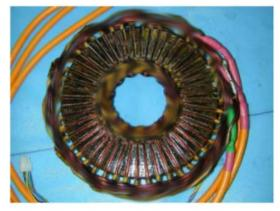
Fig 4. Stator of 195 mm od. axial flux machine
