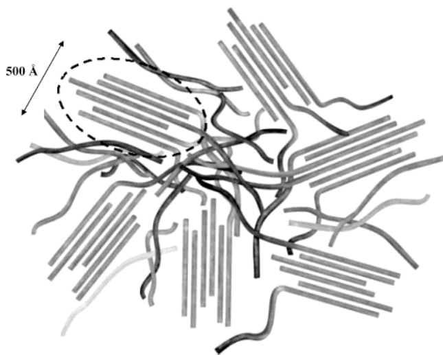
Figure 8. Schematic representation of an entangled network of elongated rodlike aggregates in Nafion. Long-range heterogeneities arising from bundles of locally ordered aggregates are proposed to give rise to the low angle increase in scattered intensity. (Reprinted with permission from the original author.)
