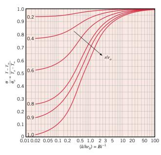
**FIGURE 5S.8** Temperature distribution in a sphere of radius  $r_o$  [1]. Used with permission.
