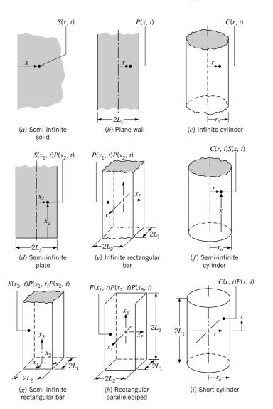
**FIGURE 58.11** Solutions for multidimensional systems expressed as products of one-dimensional results.
