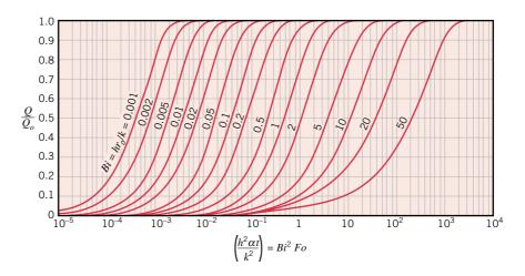
**FIGURE 58.6** Internal energy change as a function of time for an infinite cylinder of radius  $r_o$  [2]. Adapted with permission.
