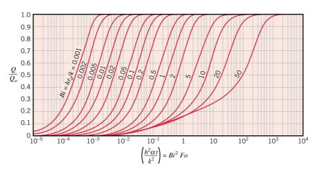
**FIGURE 5S.9** Internal energy change as a function of time for a sphere of radius  $r_o$  [2]. Adapted with permission.
