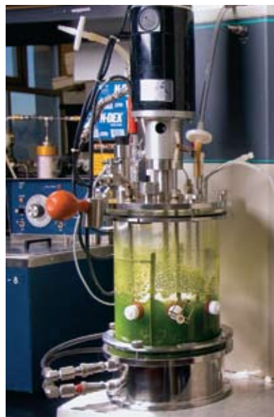
Hydrogen is produced using green algae and cyanobacteria by separating the photosynthetic protein complexes and enzymes from the cells and suspending them in solution.
