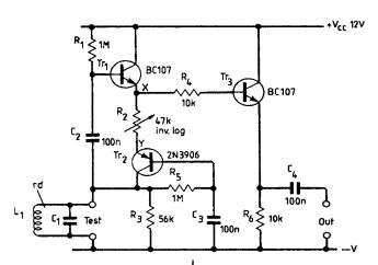
circuit under test. When R2 is set at the critical point its scale is read off in the dynamic resistance (rd) of the LC circuit.
