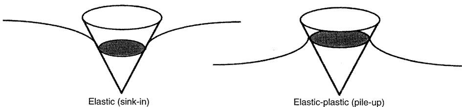
Fig. 5 Sink-in and pile-up during indentation
