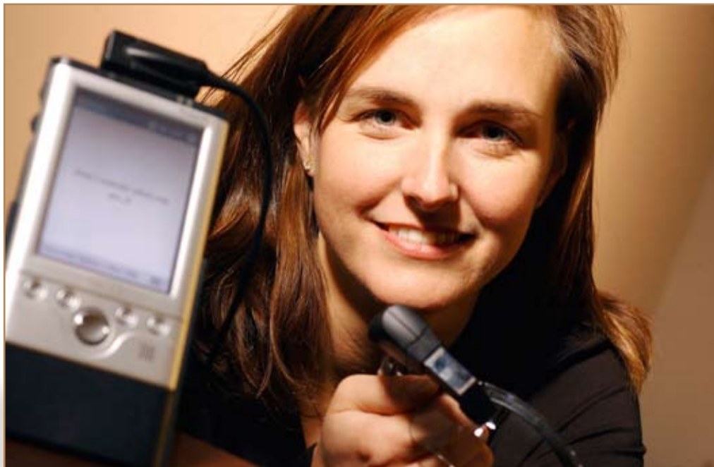
GTRI researcher Leanne West displays equipment that is part of a wearable captioning system for providing text-based information to people who are deaf or hard-of-hearing.
