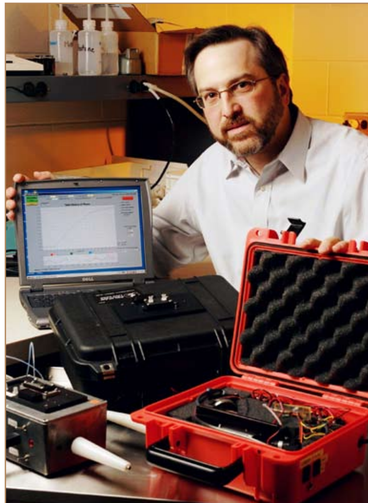
GTRI researcher David Gottfried shows components of GTRI's optical waveguide sensor, which is being evaluated as a potentially more rapid means of detecting avian influenza.
