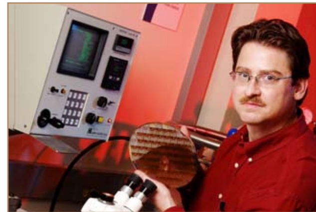
John Cressler of the Georgia Electronic Design Center holds a 200-gigahertz silicon-germanium integrated circuit wafer.
