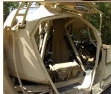
The ULTRA AP concept vehicle was built to evaluate science and technology options that could improve the design of future military vehicles. A key feature is the “blast bucket” designed to protect crew members.
