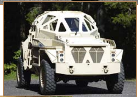
The ULTRA AP concept vehicle was built to evaluate science and technology options that could improve the design of future military vehicles. A key feature is the “blast bucket” designed to protect crew members.
