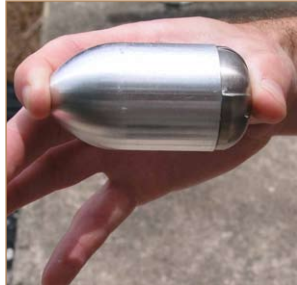
The Self Correcting Projectile for Infantry Operation (SCORPION) uses tiny microjets known as synthetic jet actuators to make mid-course corrections for improving the projectile’s accuracy.
