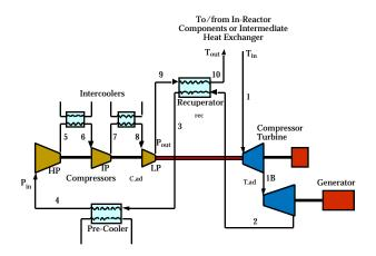
Fig. 1 Brayton Cycle as ideally applied to fusion power plant
