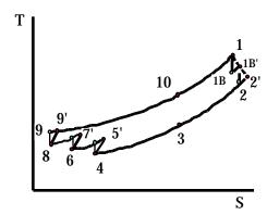
Fig. 2 Typical temperature-isentropy (T-S) plot for Brayton cycle shown in Fig. 1
