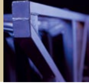
Stainless steel under the skin. The exhaust system and the SCR muffler are made of stainless steel. The Volvo 8500 with 12-litre engine also has a frame made of stainless steel.
