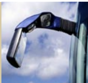
Large glass panels and rear-view mirrors. Large glass panels and three-section rear-view mirrors with integrated close-quarter mirrors provide good all-round visibility.
