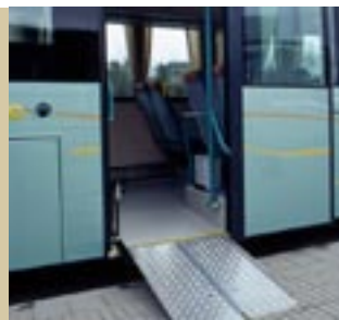
Low entry and boarding ramp. Boarding height at the front door of the Volvo 8500 Low-Entry is 320 mm and this can be lowered a further 70 mm with the kneeling function. The Volvo 8500 Low-Entry can be equipped with a wheelchair ramp.
