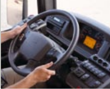
An entirely new instrument panel with large and clear instruments, a convenient display for driver information and logically grouped controls beside the steering wheel.
