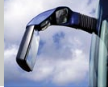
Three-section rear-view mirrors with integrated close-quarter mirrors provide excellent all-round visibility.
