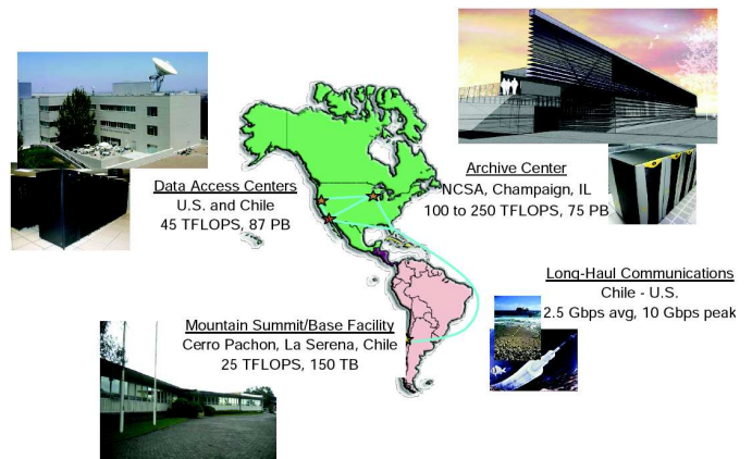
FIG. 17.— The LSST data flow from the mountain summit/base facility in Chile to the data access center and archive centers in the U.S.
