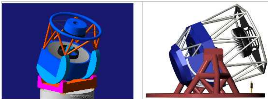
Fig. 24.— 8.4m LSST Alt-Az Telescope concepts. At left is a dual “C” ring concept similar to the LBT and MMT, by Davison (UA, Steward Observatory). The right panel shows a concept based on a more-traditional fork configuration by Claver and Muller (NOAO).
