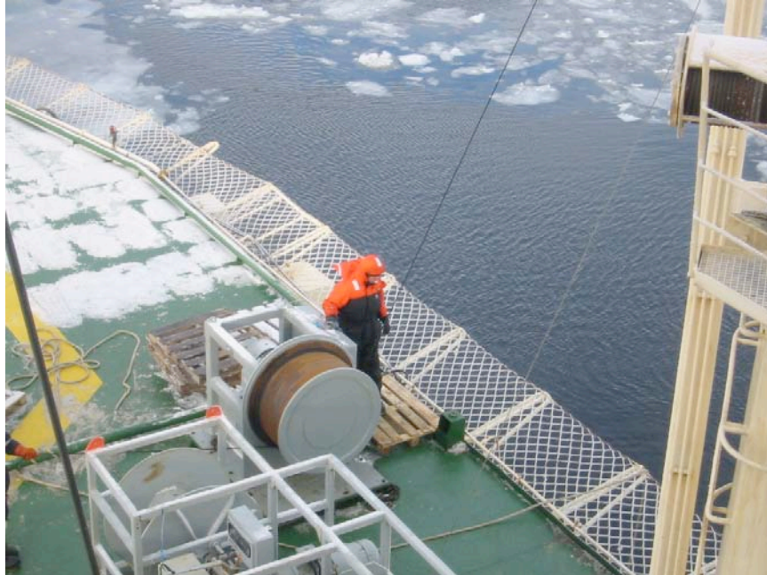
Figure I.2.3: HAWBOLDT C15-40 horizontal capstan on the helicopter deck of I/B "Kapitan Dranitsyn" (photo by Robert Chadwell, IARC).
