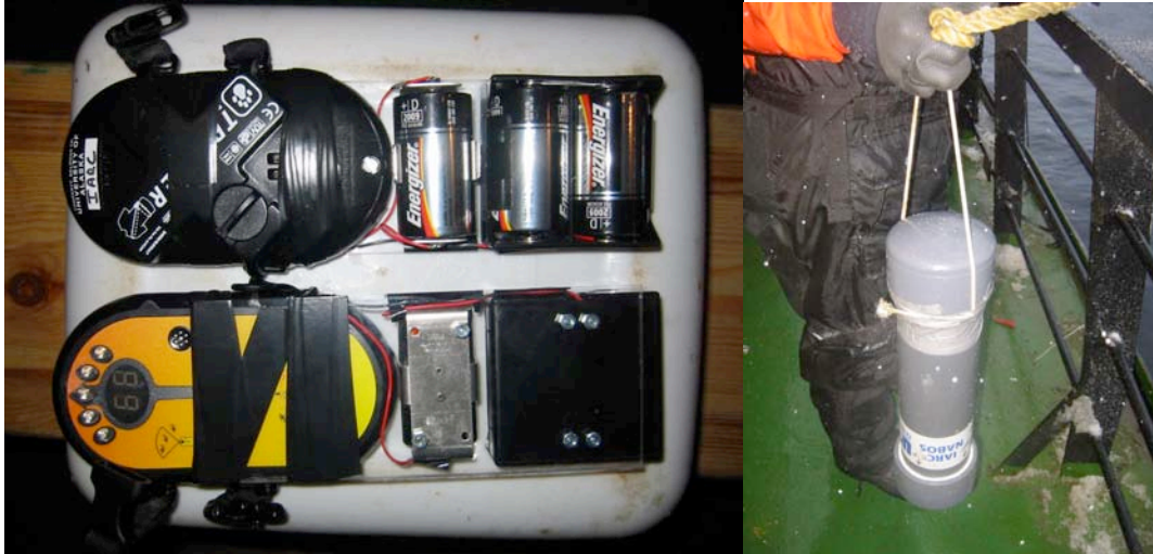
Figure I.7.3.16: Beacon (left) and beacon placed in a heavy gauge Schedule 80 PVC housing with rounded slip caps (right).
