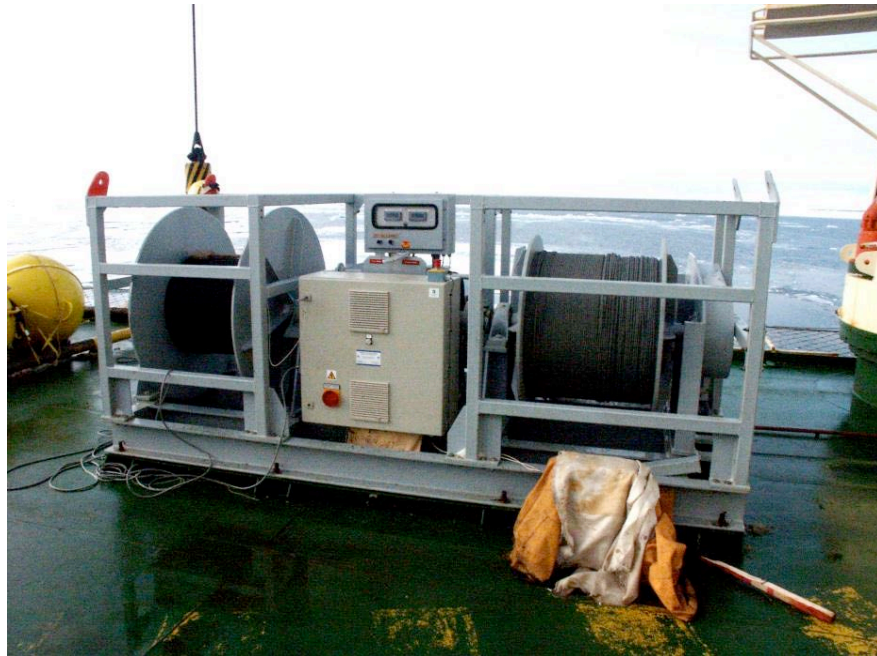
Figure I.2.2: LEBUS double-drum oceanographic winch on the helicopter deck of I/B “Kapitan Dranitsyn” (photo by Robert Chadwell, IARC).
